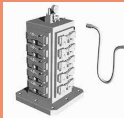
Blank system + hydraulics. Decoupled system, typical in FMS systems.
