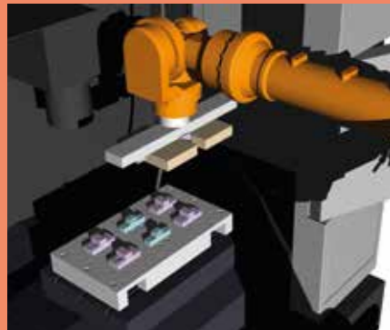
Grid System + hydraulics. Live system in vertical machining center.
